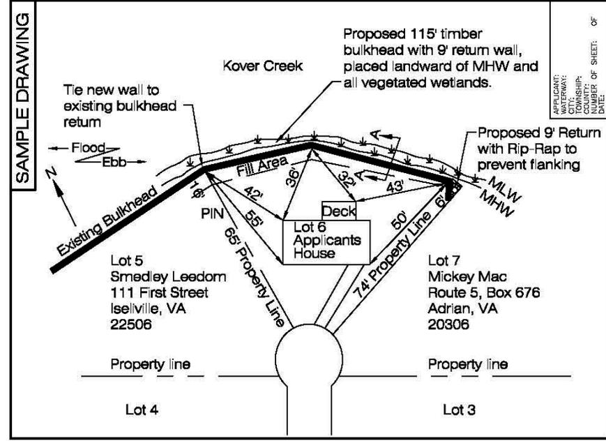
Bulkheads and Associated Backfill
