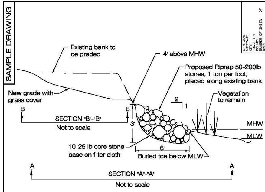
Riprap Revetment & Associated Backfill
