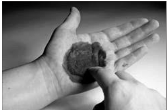
Figure 2. Step 2: Take a pinch of soil from your texture ball. Place it in the palm of your hand, and add water. Rub the soil
